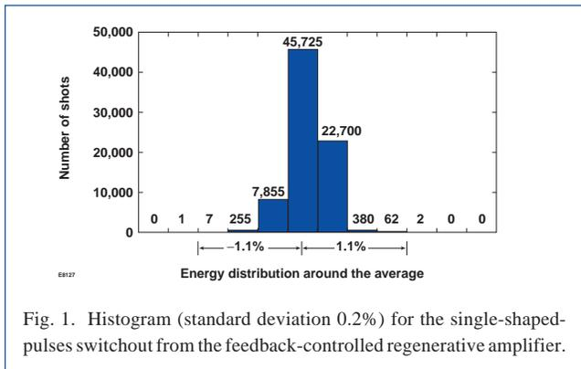
Fig. 1. Histogram (standard deviation 0.2%) for the single-shaped-pulses switchout from the feedback-controlled regenerative amplifier.
