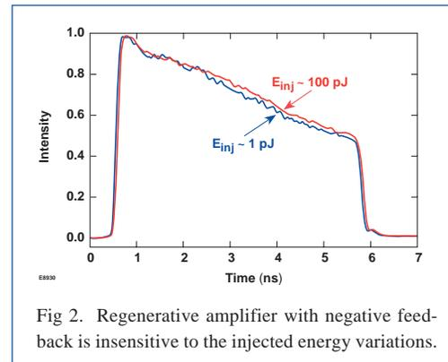
Fig 2. Regenerative amplifier with negative feedback is insensitive to the injected energy variations.
