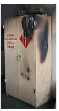
All flammable solvents in excess of the 3-gal. limit must be stored in approved flammable solvent storage cabinets
