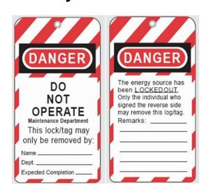
Lockout/Tagout (LOTO) – prevents operation of equipment that could cause injury or equipment damage. LLE instructions 6300 defines LLEspecific LOTO procedures
