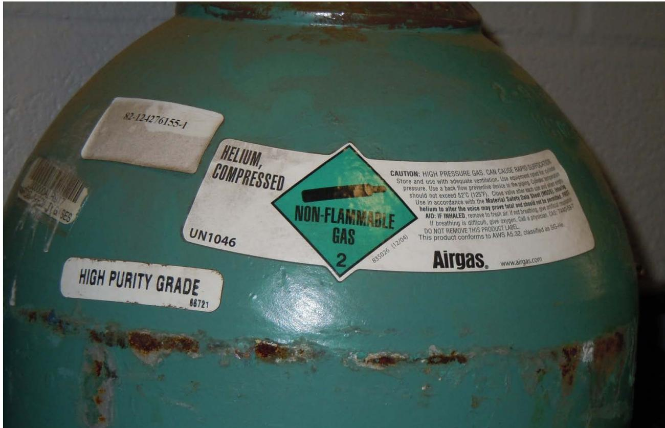
**Cylinders that do not have a legible label must not be used and must be returned to the gas supplier**
