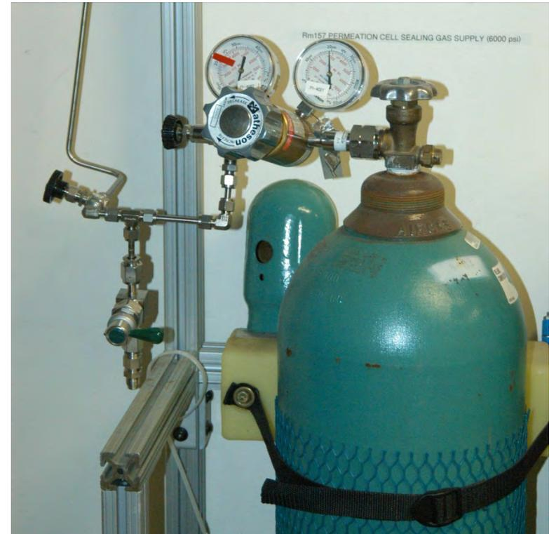
**Vacuum fittings are not to be used on pressurized gas systems unless they are specifically rated for pressure applications**
