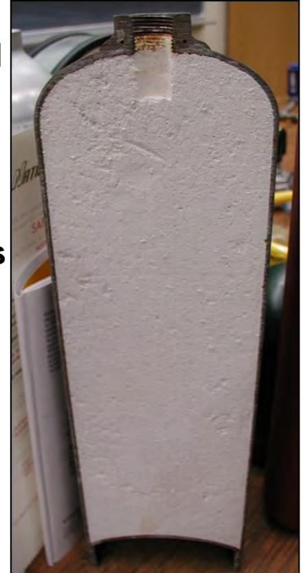
**Acetylene cylinders must always be stored upright. If a cylinder is lying on its side, it must be stored upright for at least 30 minutes prior to use.**
