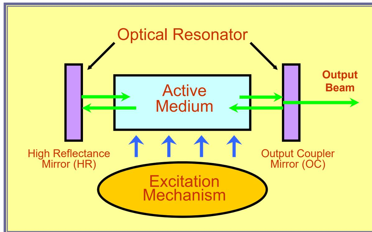
**Active medium:** This can be a solid (crystal), semiconductor (diode), liquid (dye), or gas, which contains atoms that can emit light by stimulated emission. Also known as **lasing or gain medium**
