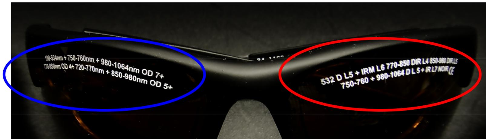
**All LLE signs use the ANSI standard with wavelength called out in nanometers (nm)**
