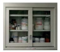
Flammable solvent storage outside of an approved storage cabinet is limited to 8 gallons per "fire area"
