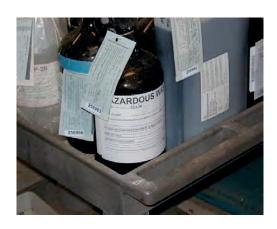
Secondary containment required to control spills or container leaks
