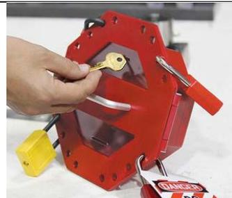
Figure 3 - A group lockbox is used for multi-point lockout, or when a lockout device is not capable of supporting multiple locks.
