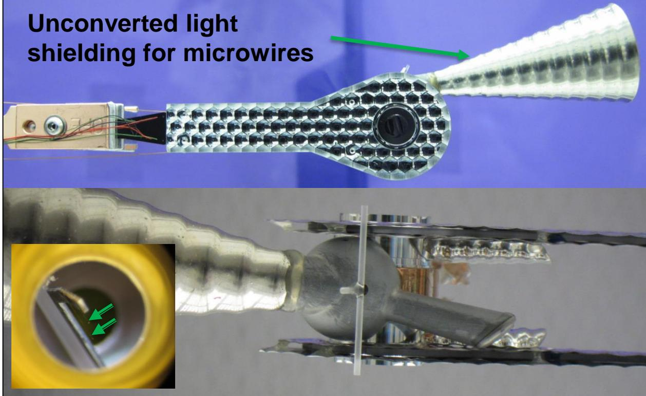
Platform facilitated first imaging using ARC illuminated microwire backlighter with full hohlraum and backlighter shielding and apertures
