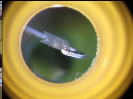
V-shaped plasma mirrors were used to increase the ARC energy that is incident on the 25um microwires
