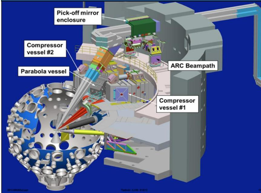
Used to produce Bremsstrahlung X-ray backlighter sources over the range of 50 keV-200 keV
