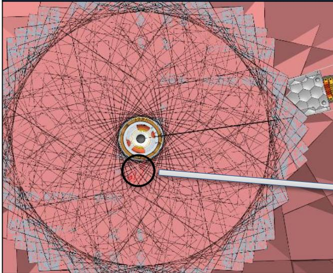
$1\omega$  unconverted light starts at 4.75 mm radius and extends to 37.5 radius
