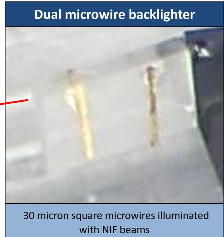
Several backlighter only targets were designed and fielded to test wires at the bottom plastic V-shaped grooves to help get more laser energy on the wires.
