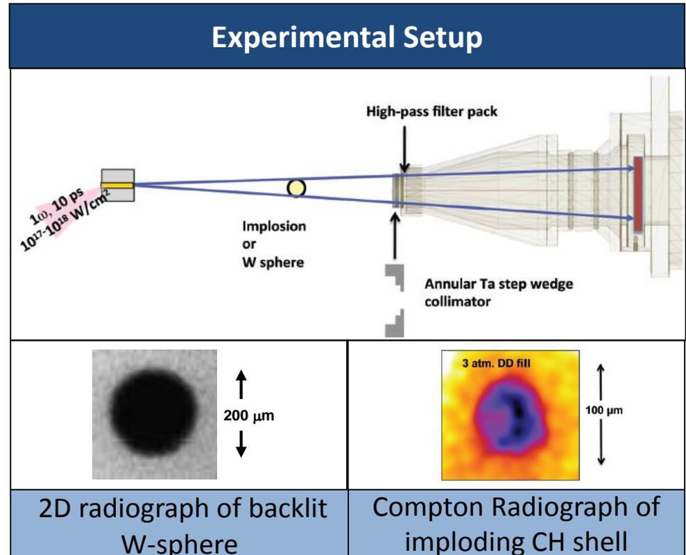
Relatively simple targets could be built and many experiments could be run to test backlighter energy and resolution (See Kelly Youngblood's poster)
