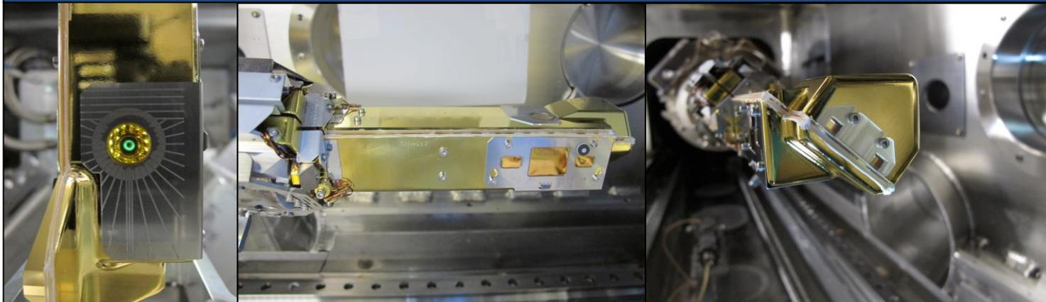
Shroud validated with an existing layering target retrofitted with ARC shield
