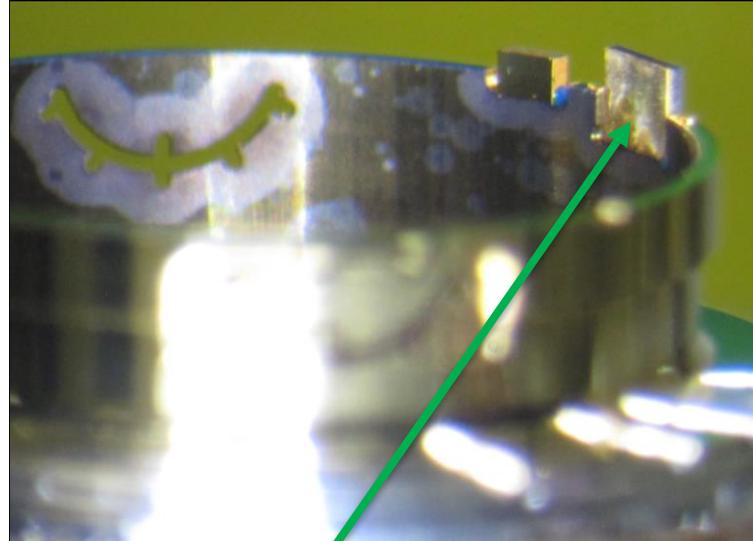
15 micron thick gold foil bonded to standard hohlraum diagnostic windows will confirm Compton platform imaging capability
