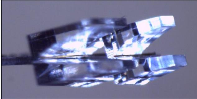
Higher resolution 10 micron diameter microwires with parabolic plasma mirrors
