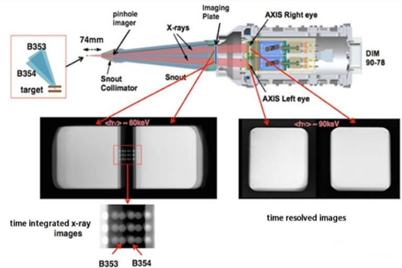
Provides high detection quantum efficiency at the 40-200 keV x-ray range required for Compton radiography
