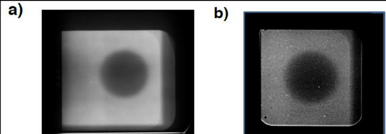
Au microwire backlighter, recorded on Image Plate, a), and on one of the two AXIS framing cameras, b). Credit: Riccardo Tomassini
