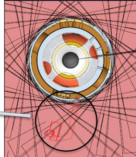
Compton radiography backlighter is completely within the unconverted light and must be shielded to mitigate preheating of the backlighter microwires
