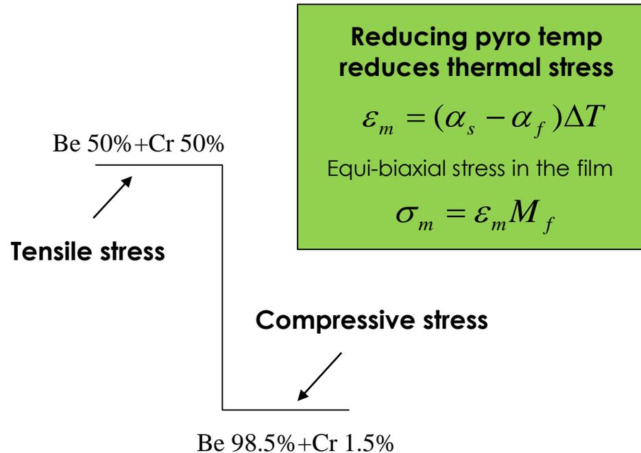
At pyrolysis temperature, thermal stress:
