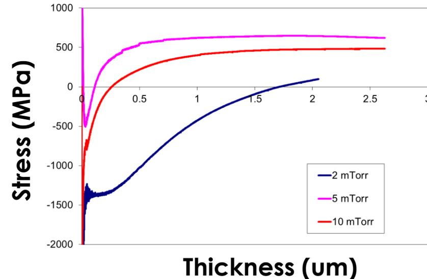
Cracking happened in S-curve region where both deposition and thermal stress are high whereas mostly amorphous structure is weak
