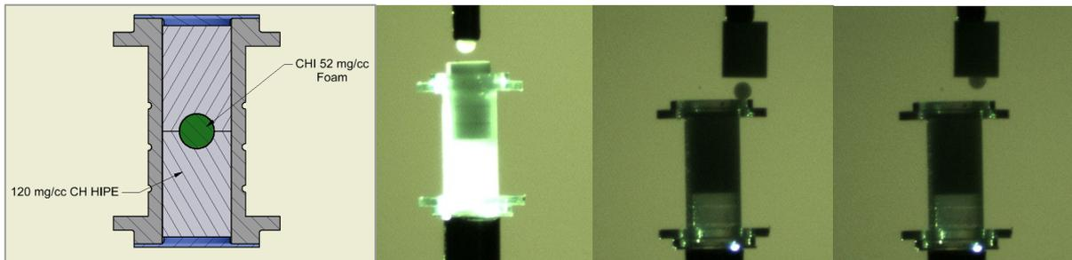
Void collapse target and robotic assembly of foam void
