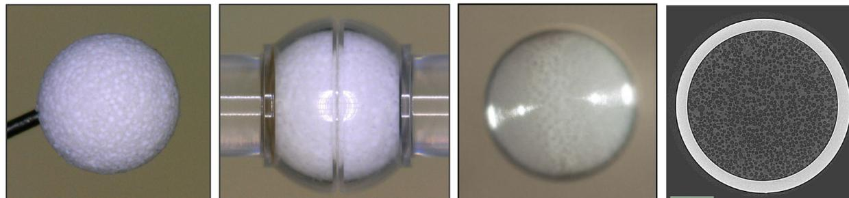
The engineered foam sphere is stuffed into the CH ablator and back machined before tomography
