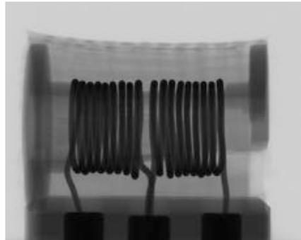
Zylon-wrapped coil is intact after a 31T shot. 58T achieved to date (~70T max)
