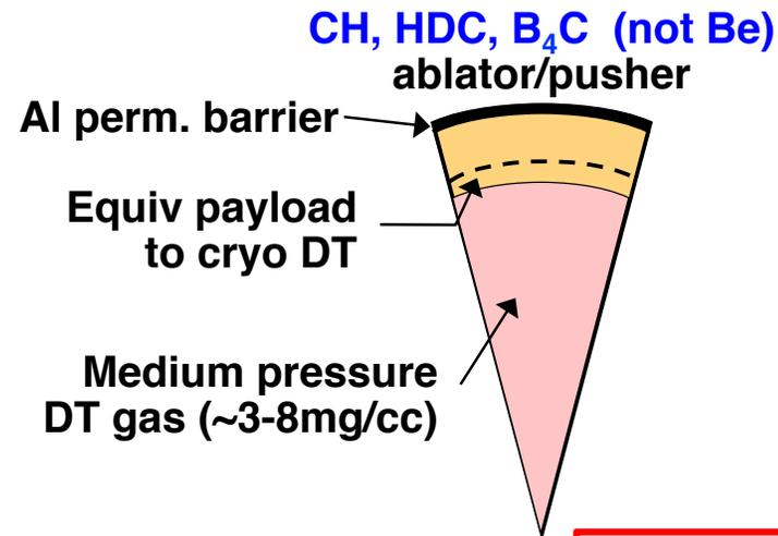
Room-temp gas capsules for proof-of-principle tests
