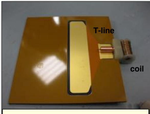
Zylon wrapped coil and T-line
