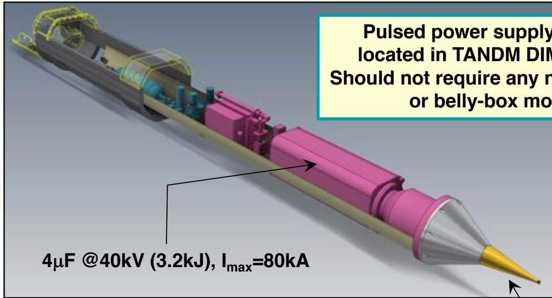
Room-temp hohlraum coil for first set of gas-target shots.
