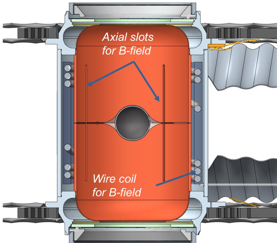
Wire wrapped on the inside of the diagnostic band
