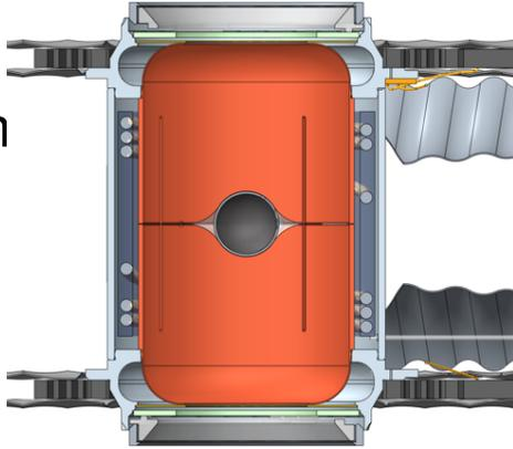
Ramping the current in the coil creates a voltage across the slots. Assume 4 slots of 100  $\mu\text{m}$  width:
