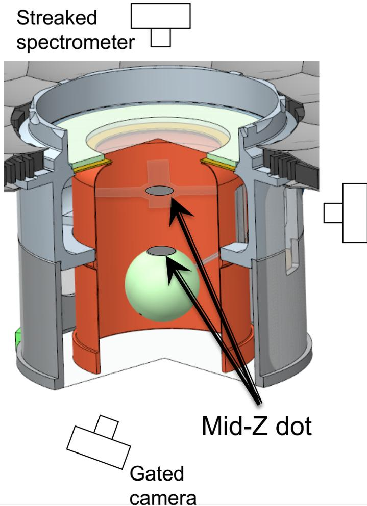
Te measurements can be made using mid-Z tracer spectroscopy or optical Thomson
