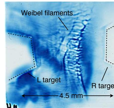
Proton radiograph from OMEGA EP,  $t = 4.8$  ns [1]
