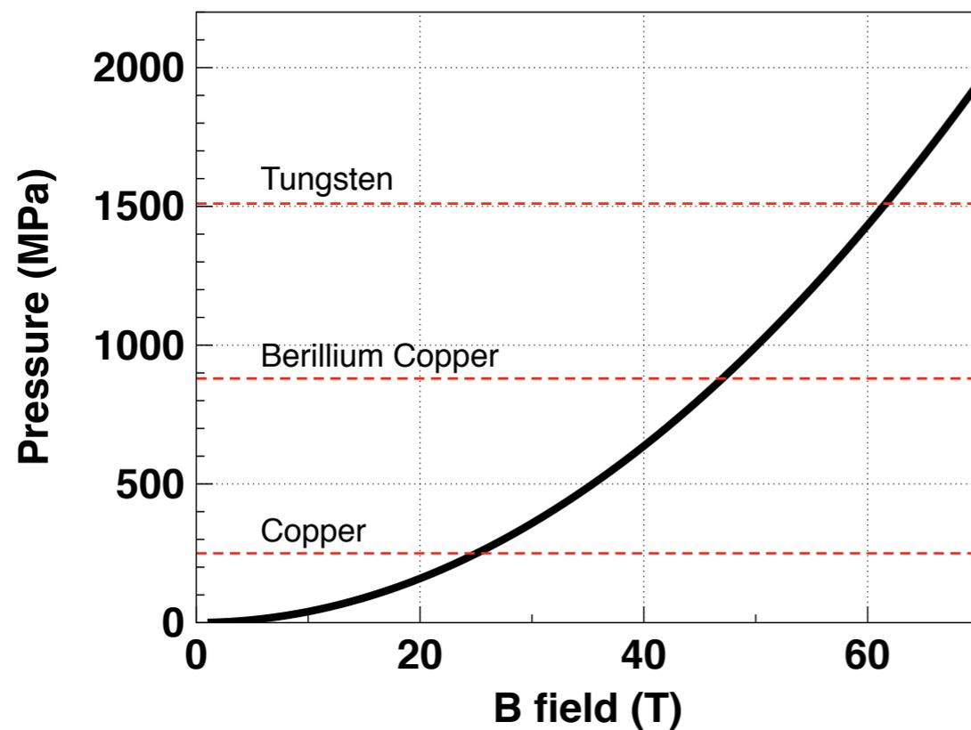
Coil displacement becomes very large destroying the structural integrity
