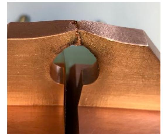
**With a stronger material, a field as high as 40 T could have been possible. E.g. Beryllium Copper is x3 stronger while still low-resistive.**
