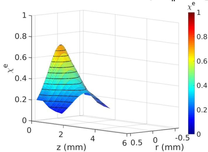
$$q_r^e = -\chi_{\perp}^e \frac{\partial T_e}{\partial r} \quad q_z^e = -\chi_{\parallel}^e \frac{\partial T_e}{\partial z}$$
