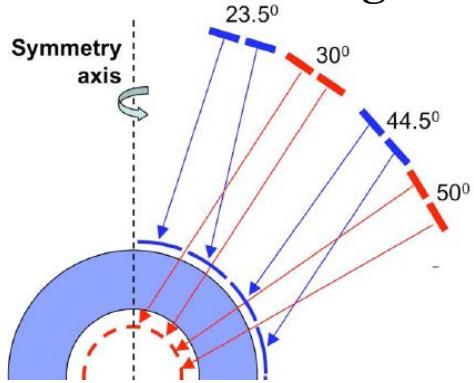
The polar-drive design for the 96 main beams has 24 pointing and focusing parameters
