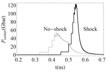
Re-shock technique with one shock (for a given shock strength)
