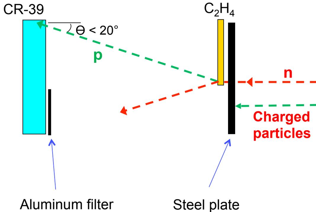
Proton energy will be determined based on track size on the CR-39
