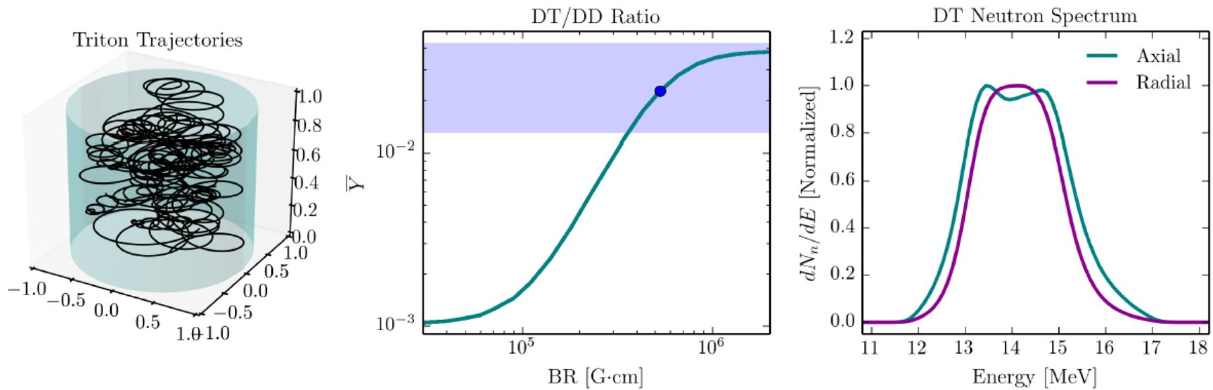
The pre-imposed  $B_z$  field magnetizes the plasma trap the tritons and direct them axially in helical orbits.
