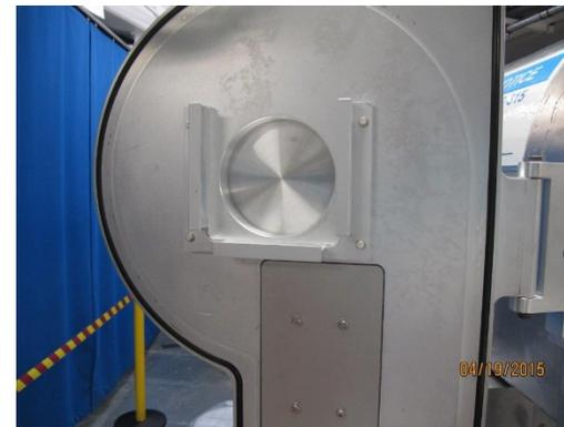
An inexpensive neutron detector, consists of a stack of polyethylene converter in front of an image plate. We have been looking at the performance of this system for imaging of high yield experiments.
