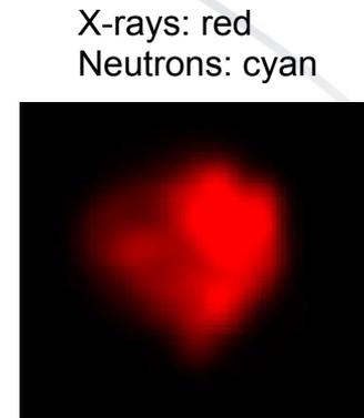
A comparison of neutron images to x-ray images shows significant differences due to uneven distribution of mix in the simulations.
