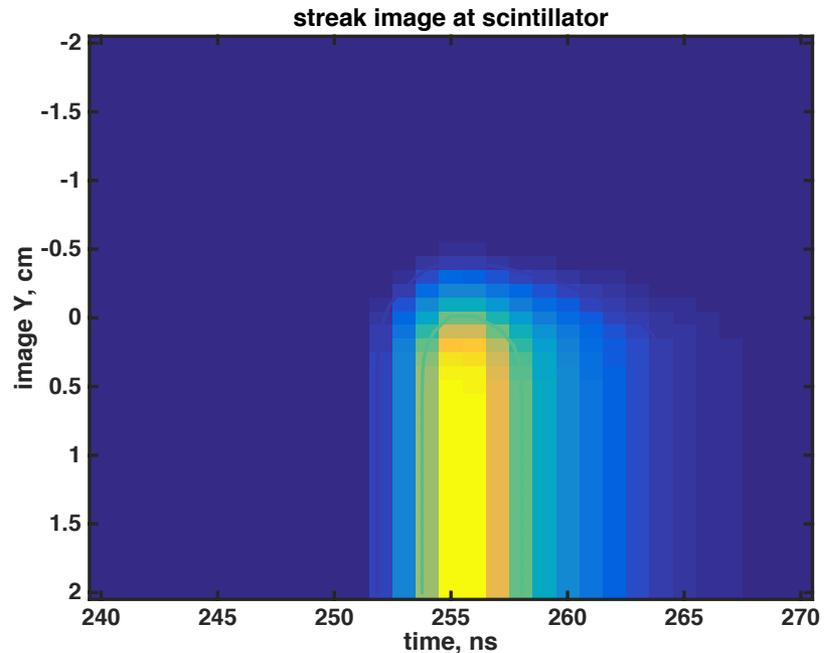
Simulated streak image for 200x magnification rolled edge, 1D simulated source plasma with  $T_{ion} = 4$  keV (avg)
