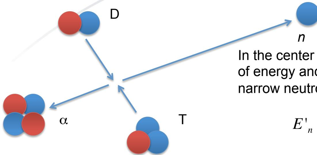
In the center of mass frame, conservation of energy and momentum results in a narrow neutron energy spread.
