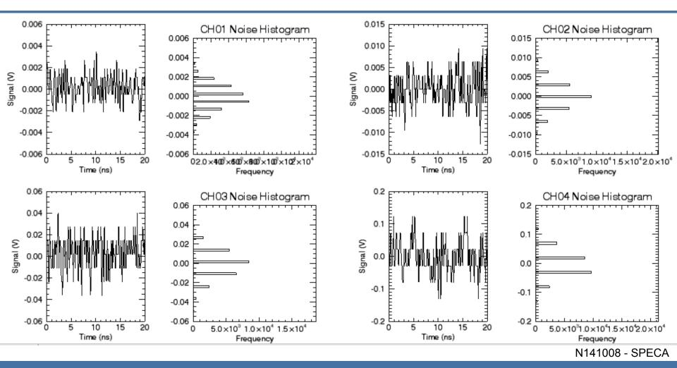
Typical scope noise floor is normally distributed and accounts for 5-7 ADC points
