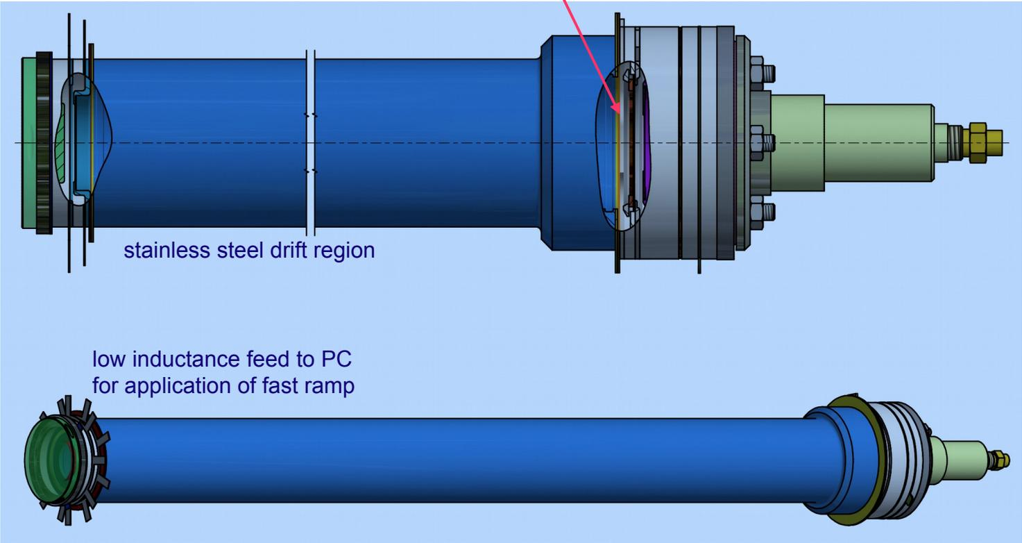
low inductance feed to PC for application of fast ramp
