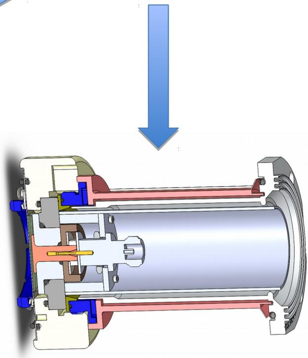
ground arrangement not ideal and resulted a in 0.5 GHz oscillation
