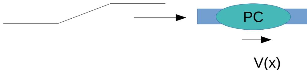
at a given instant there is a voltage gradient along the cathode
