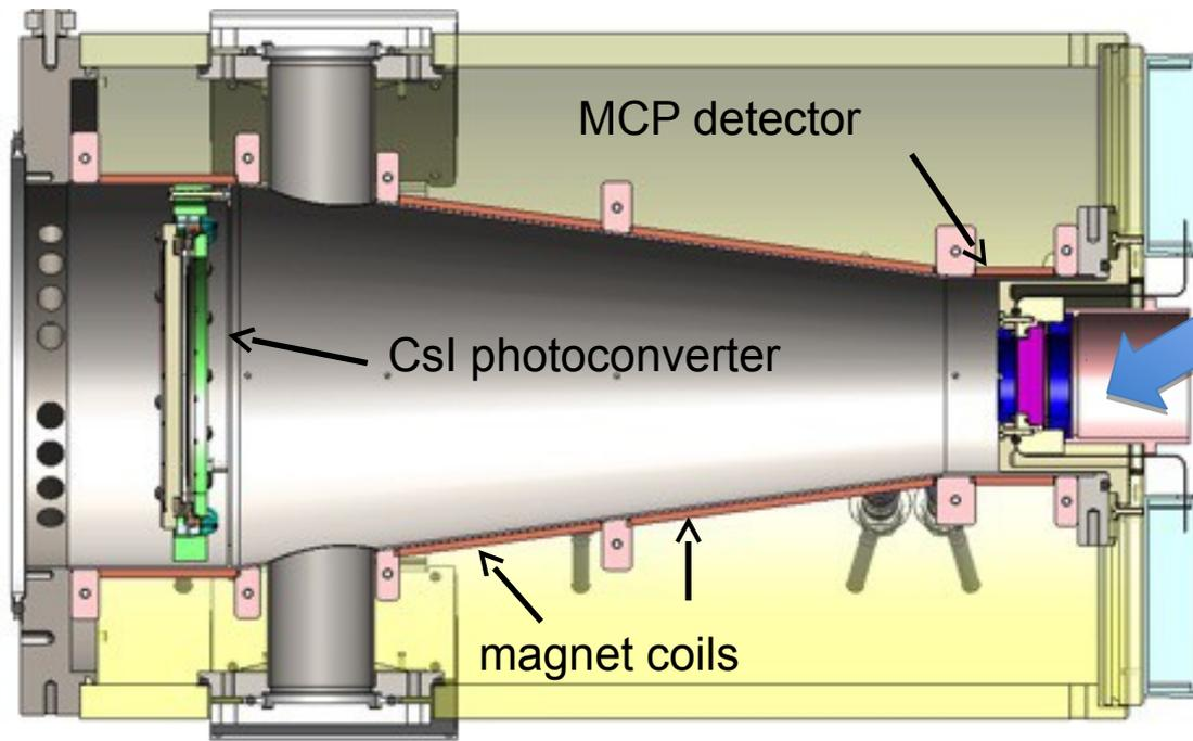
phosphor window replaced with collection anode with N-type coaxial connector
