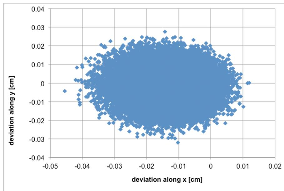
Here effect contributes  $\sim 100 \mu\text{m}$  to electron spreading, about same as that due to electron birth energy of 1.7 eV
