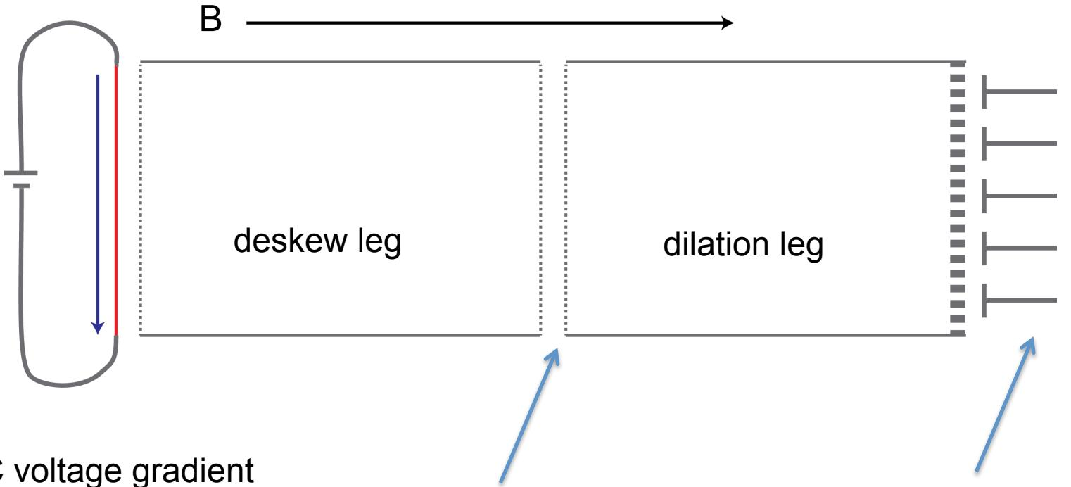
DC voltage gradient applied at cathode. Resulting velocity dispersion removes skew after appropriate drift distance.
