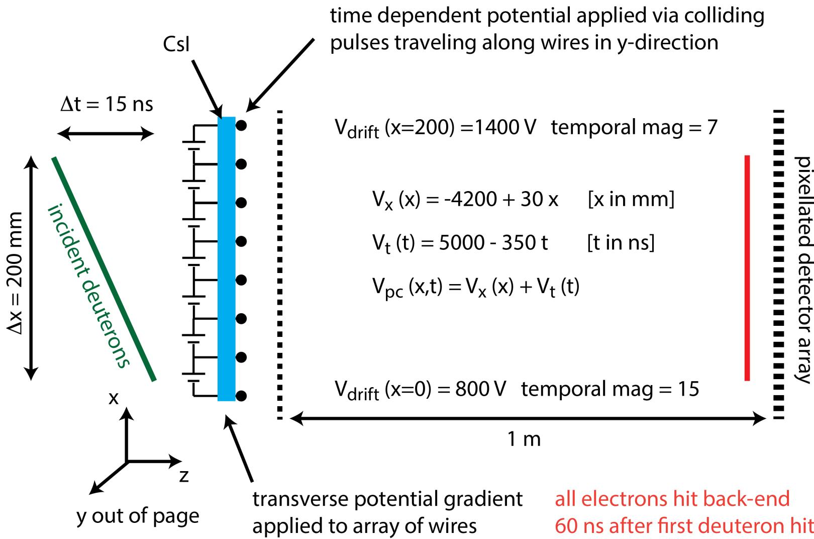
*a concern is the  $E_x$  in acc. gap and its effect on electron orbits*
