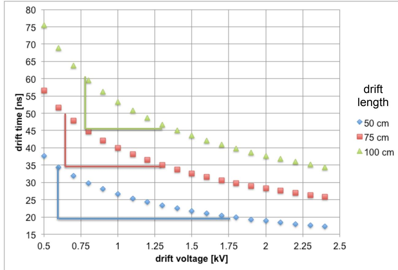
**15 ns skew can be removed using 800-1400V drifts over a meter**
