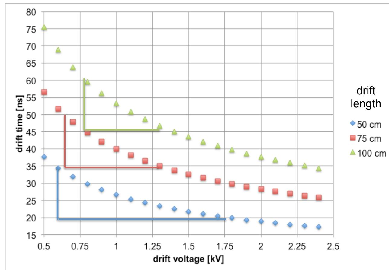
15 ns skew can be removed using 800-1400V drifts over a meter
