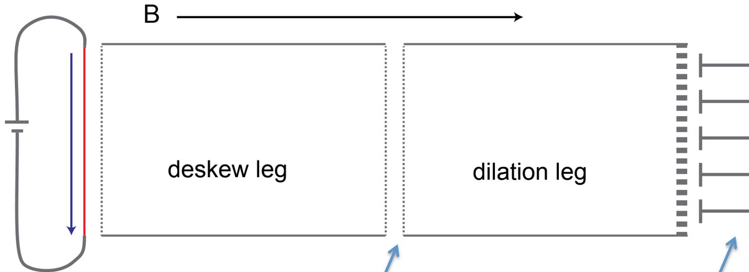
DC voltage gradient applied at cathode. Resulting velocity dispersion removes skew after appropriate drift distance.
