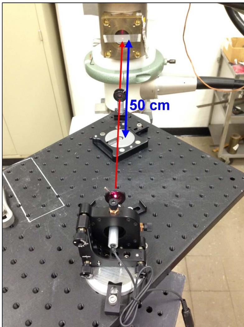
Crystal alignment: The crystal is mounted on a precision rotation stage and is rotated to the Bragg angle + (301) asymmetric angle  $\Theta_B + \Theta_A$ . The slit and IP holder are aligned to the red beam reflected from the back of the crystal when rotated by the Bragg angle  $\Theta_B$ :
