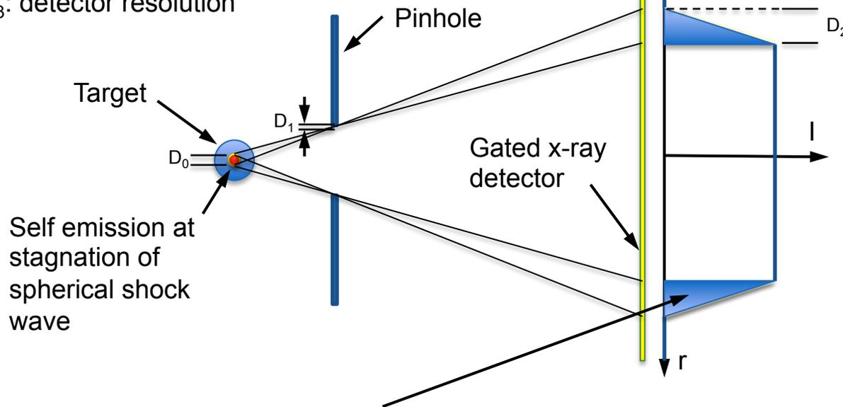
Self emission at stagnation of spherical shock wave
