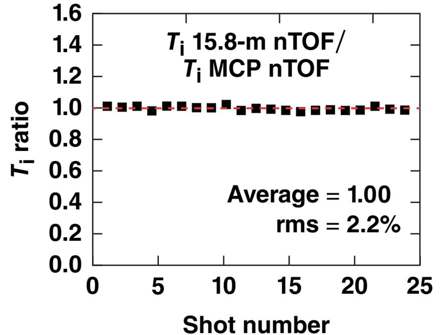
The MCP nTOF is a promising detector for  $T_i$  measurements.
