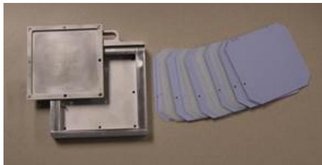
An inexpensive neutron detector, consists of a stack of polyethylene converter in front of an image plate. We have been looking at the performance of this system for imaging of high yield experiments.
