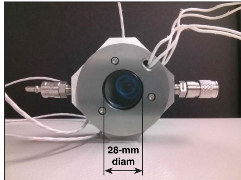
**The CLBO crystal is enclosed in an oven with dry nitrogen and held at 120°C to avoid hygroscopic damage to the surfaces.**
