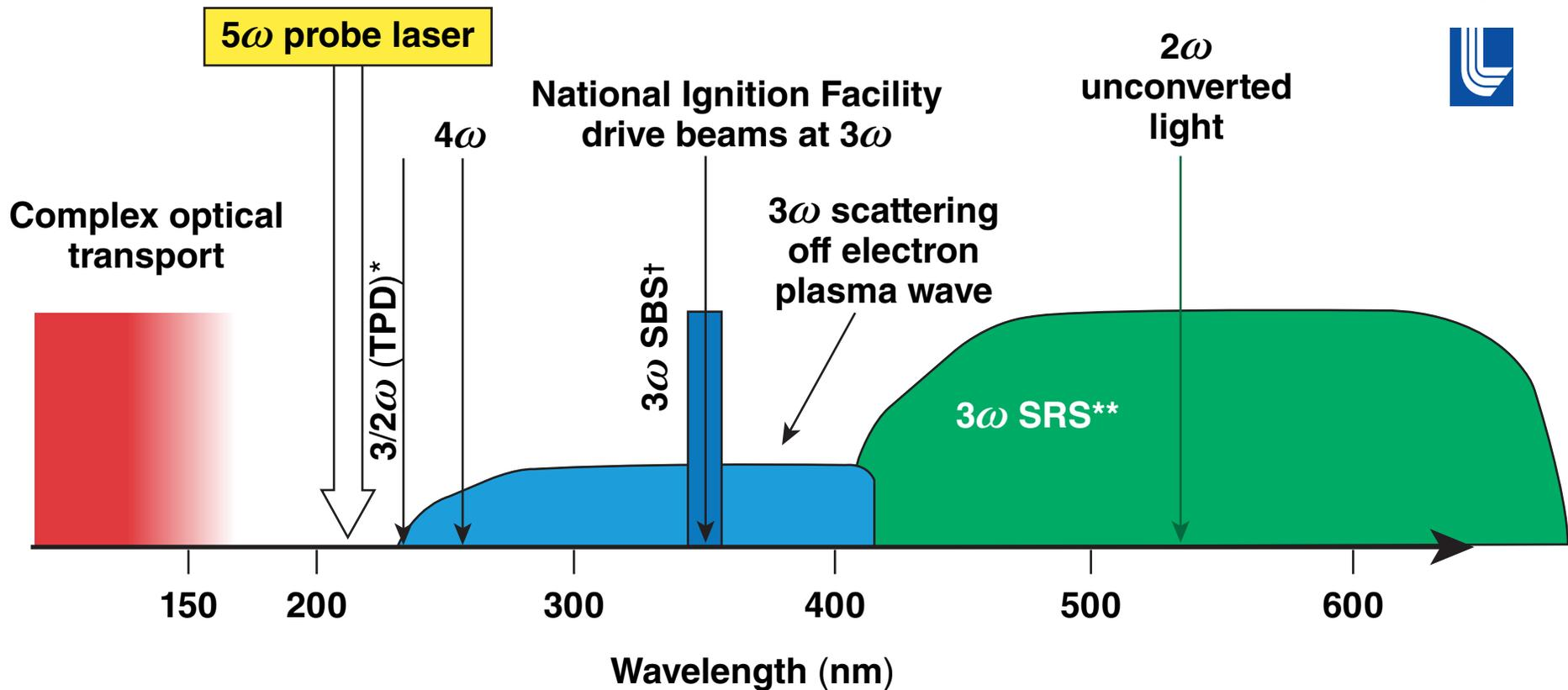
Frequency conversion of a 100-J, 1053-nm laser to the fifth harmonic is required to produce 10 J at 211 nm.
