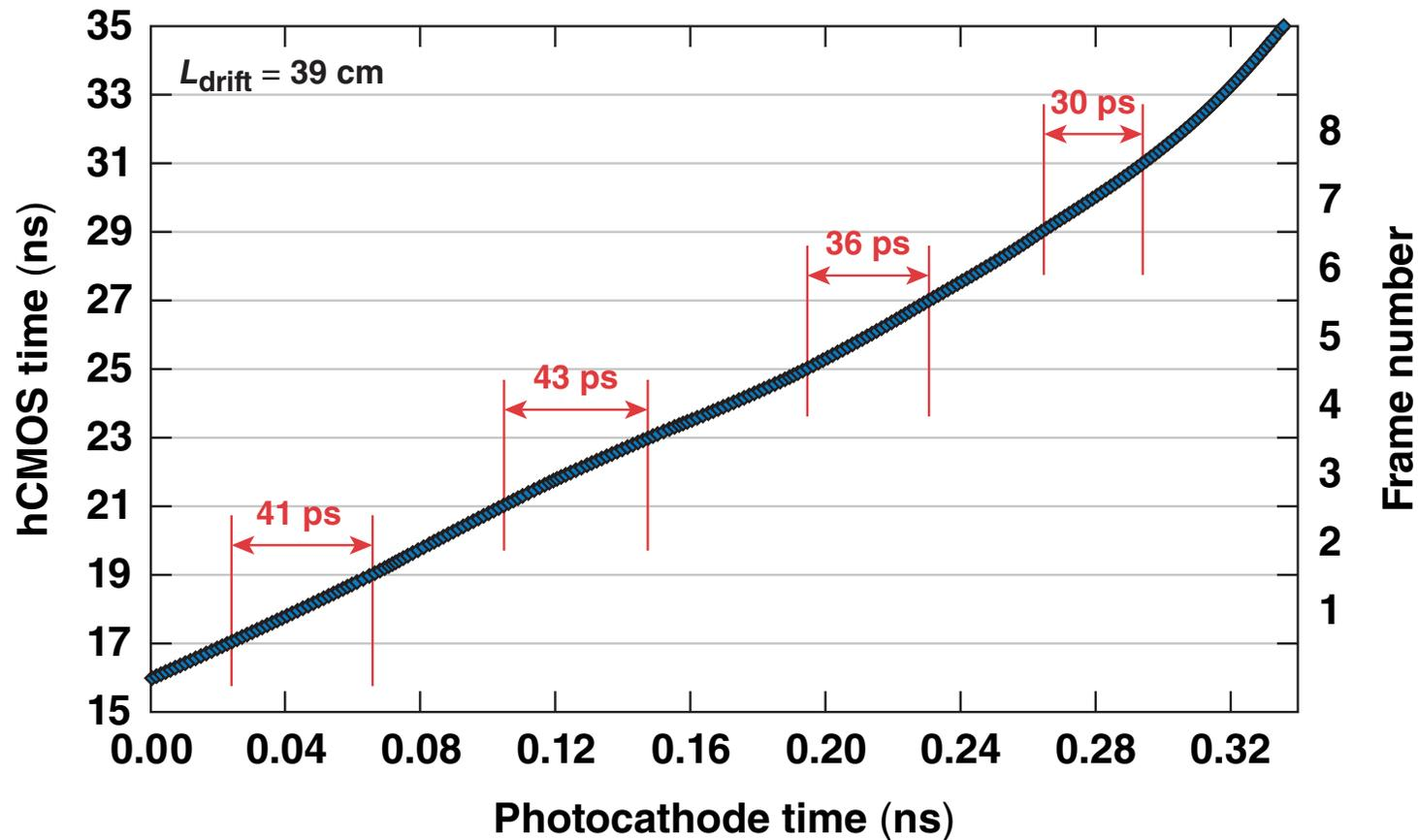
A 50-cm drift tube will be developed that will provide ~30-ps time resolution.
