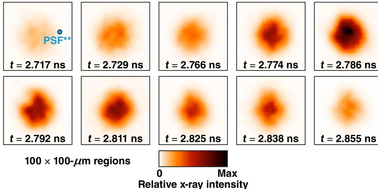
KBframed has 30-ps temporal resolution and 6- $\mu\text{m}$  spatial resolution, and records an image every 15 ps in the 4- to 8-keV photon-energy range.
