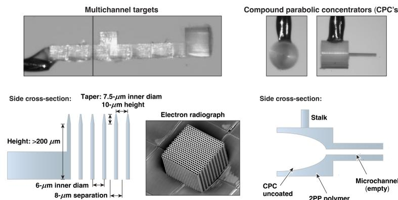
We have developed two target designs to increase the efficiency of coupling with a microchannel. Multichannel targets use about 400 microchannels arranged in a close-packed hexagonal array in order to maximize the likelihood of laser light entering one or more channel openings. Compound parabolic concentrator targets use a flared opening to reflect misdirected laser energy into a single channel.
