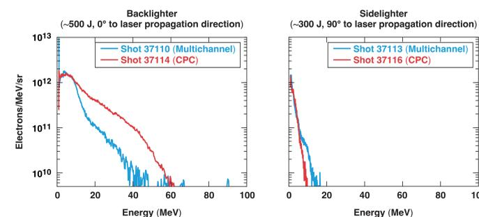
For backlighter and sidelighter shots, respectively, the EPPS was positioned at 0° and 90° relative to the axis of laser propagation. The results indicate that relative to the multichannel targets, the CPC targets produced more energetic electrons in the forward direction, but fewer energetic electrons orthogonal to laser propagation. This suggests that the CPC targets accelerate electrons more effectively.
