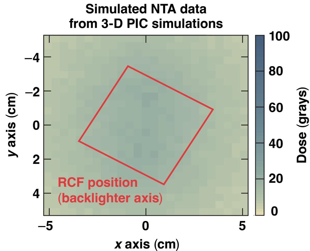
We ran a 3-D PIC simulation of a laser with the same parameters as an OMEGA EP short-pulse beam entering a 40- $\mu\text{m}$  channel filled with a 1  $n_c$  density foam with 100- $n_c$  density walls. We show a plot of the fluence of electrons above 3.5 MeV produced by this interaction, projected onto a plane 9 cm away from target chamber center for comparison with our NTA data. The size of an NTA film pack is shown in red.
