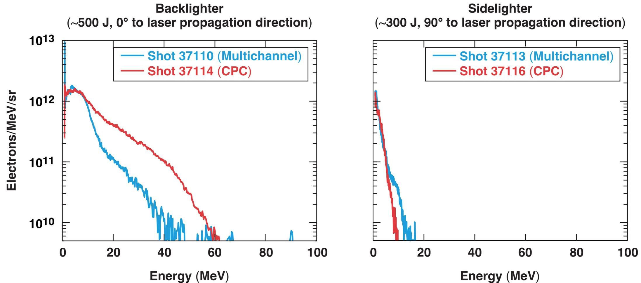
For backlighter and sidelighter shots, respectively, the EPPS was positioned at  $0^\circ$  and  $90^\circ$  relative to the axis of laser propagation. The results indicate that relative to the multichannel targets, the CPC targets produced more energetic electrons in the forward direction, but fewer energetic electrons orthogonal to laser propagation. This suggests that the CPC targets accelerate electrons more effectively.
