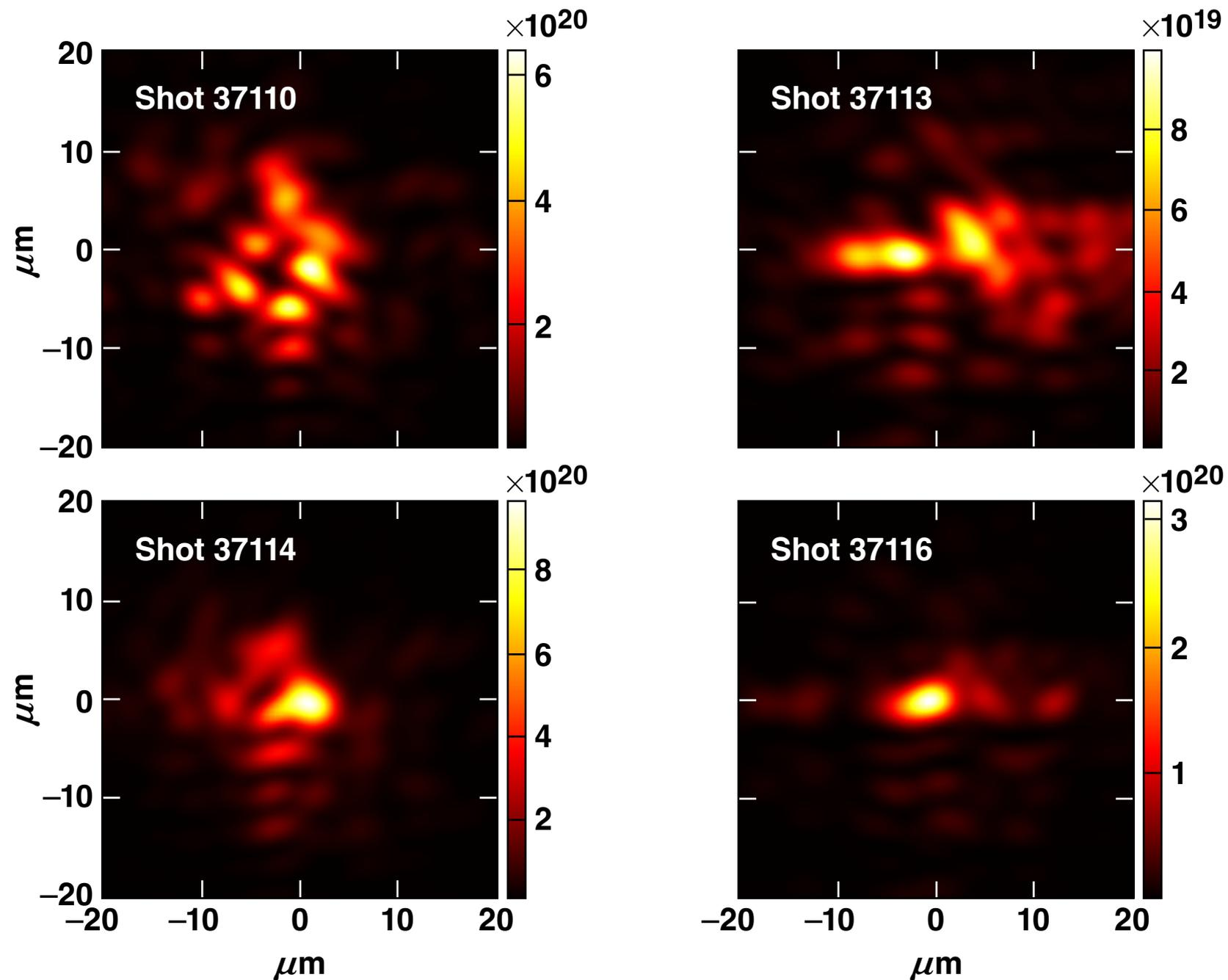
**Sending a laser pulse down a microscale tube is difficult due to shot-to-shot variability. Although the highest-intensity focus of the OMEGA EP beam (as shown above by the focal-spot diagnostic) can be smaller than  $2 \mu\text{m}$  in radius, speckles in the beam and pointing instability mean that we cannot hit a single microchannel reliably.**
