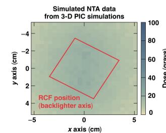
We ran a 3-D PIC simulation of a laser with the same parameters as an OMEGA EP short-pulse beam entering a 40-μm channel filled with a 1 n<sub>c</sub> density foam with 100-n<sub>c</sub> density walls. We show a plot of the fluence of electrons above 3.5 MeV produced by this interaction, projected onto a plane 9 cm away from target chamber center for comparison with our NTA data. The size of an NTA film pack is shown in red.
