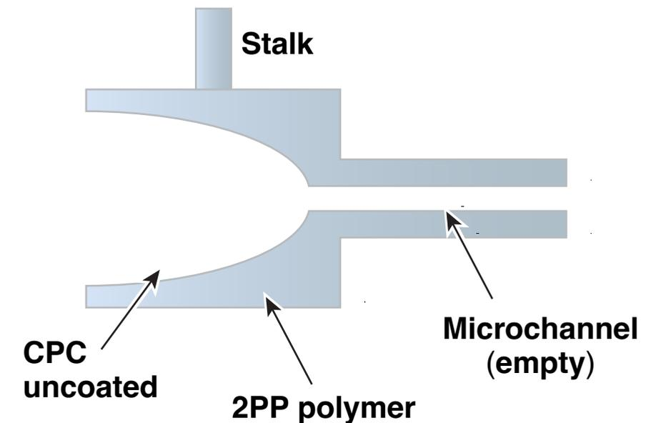
We have developed two target designs to increase the efficiency of coupling with a microchannel. Multichannel targets use about 400 microchannels arranged in a close-packed hexagonal array in order to maximize the likelihood of laser light entering one or more channel openings. Compound parabolic concentrator targets use a flared opening to reflect misdirected laser energy into a single channel.
