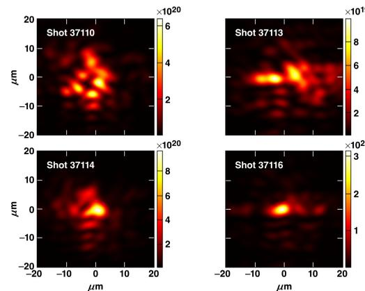
Sending a laser pulse down a microscale tube is difficult due to shot-to-shot variability. Although the highest-intensity focus of the OMEGA EP beam (as shown above by the focal-spot diagnostic) can be smaller than 2 μm in radius, speckles in the beam and pointing instability mean that we cannot hit a single microchannel reliably.
