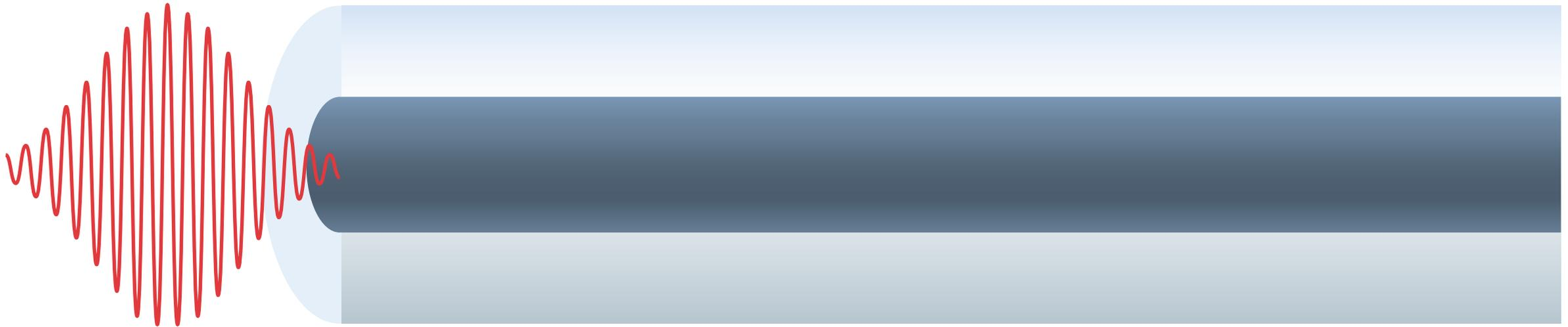
**We attempt to send a relativistic laser pulse down a micron-scale tube of overdense material. The tube may be empty or filled with relativistically underdense material. The tube acts as a waveguide through which the laser pulse propagates. During the interaction, energy from the laser pulse is transferred to electrons in the tube, which are accelerated.**
