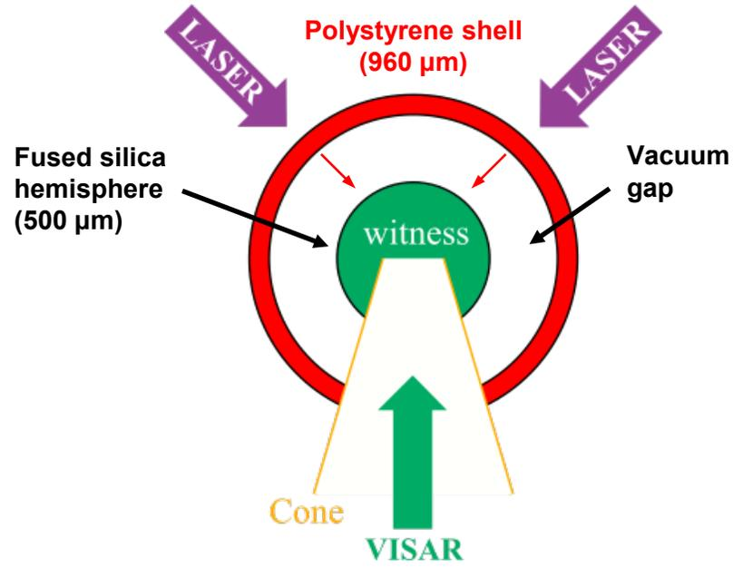
Picket pulses with varying intensity were used to drive the shock
