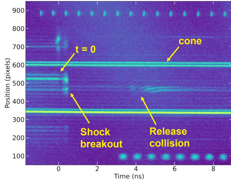
Shock velocity measurements in the witness were not affected by radiation preheat
