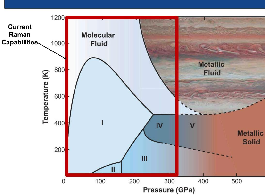
(Above) Phase diagram of hydrogen showing the predicted region of solid metallic hydrogen.[2] Raman spectroscopy for dynamic compression experiments will be used to investigate the structure of solid hydrogen above this pressure.
