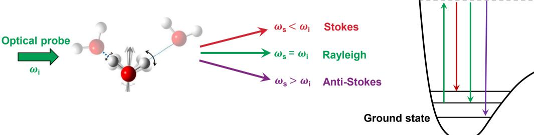
(Above) Incident photons a sample excite a sample to a virtual excited state.[1] These photons can be inelastically scattered at a different frequency based on the sample's final elementary excitation state (e.g., rotational, vibrational)
