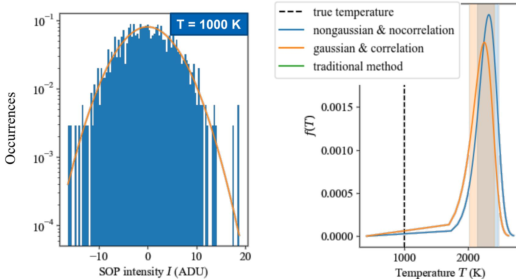
At extremely low temperatures, the traditional method run into numerical errors, while the new model at least gives us an upper bound for temperature.
