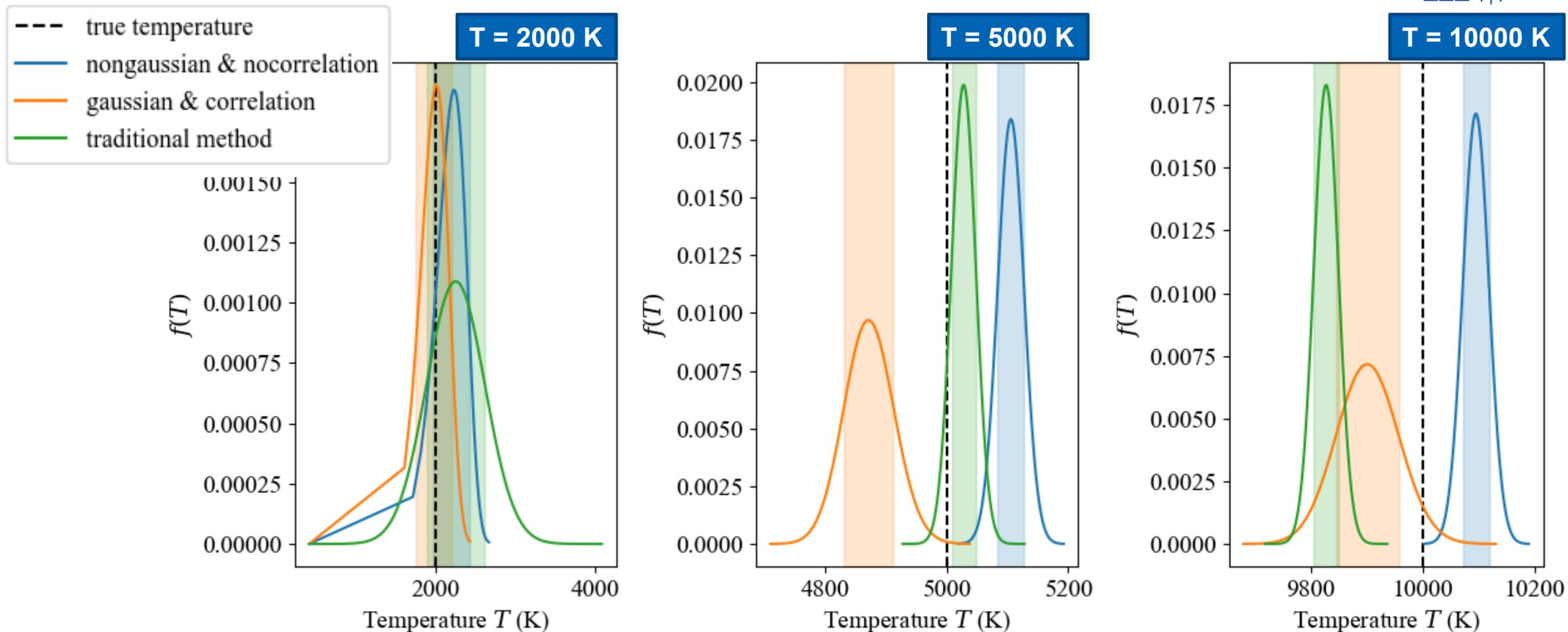
At extremely low temperatures, the traditional method run into numerical errors, while the new model at least gives us an upper bound for temperature.
