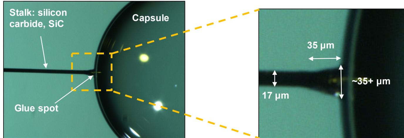
Capsule radius for OMEGA cryo targets is typically  $\sim 430$  to  $510\ \mu\text{m}$
