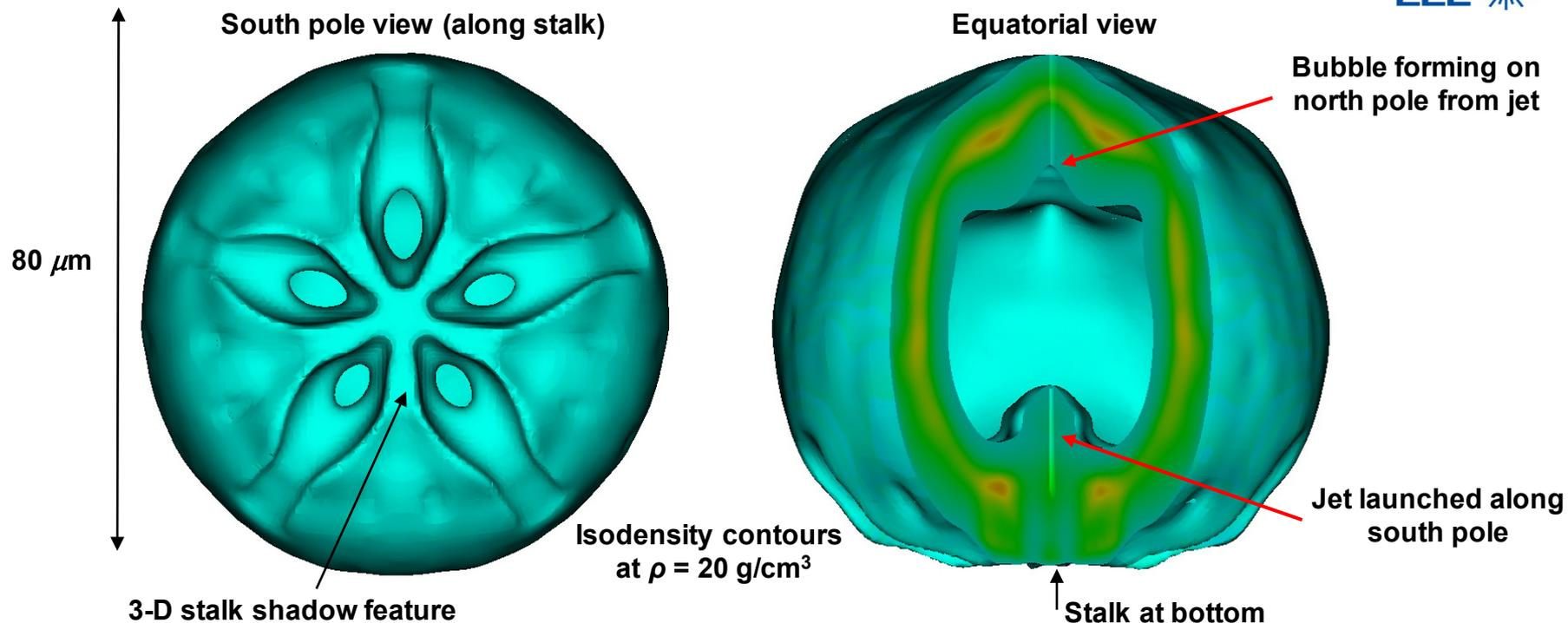
Stalk shadowing did not significantly degrade target performance
