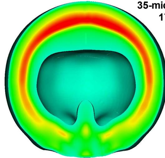
Iso-density surface at stagnation, simulated with 35-micron glue spot and 17-micron stalk
