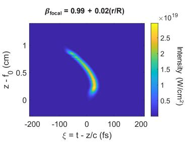
The DM-SLM pair offers rapid, tunable exploration of exotic flying foci, which improves upon the previously proposed static reflective echelon [2]. An example of an exotic focal velocity is one shown on the left. Initiating the flying focus with  $\beta_{\text{focal}}$  < 1 allows for controlled trapping of background charge: subsequent acceleration of the focus beyond  $\beta_{focal} = 1$  mitigates dark current and wave breaking.
