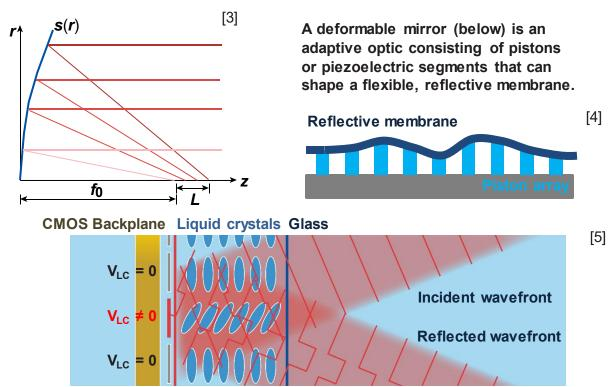
A spatial light modulator (above) consists of an array of liquid crystals (LCs). Applying some voltage  $(V_{LC})$  to a LC causes the LC to rotate. The rotation of the LCs results in changes in the local refractive index.
