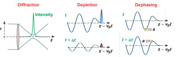
Electron dephasing can be circumvented by using custom optics to produce a flying focus: an intensity peak with a controlled velocity which sets the phase velocity of the driven wakefield [2]. This poster presents simulations of a novel optical configuration for spatiotemporal pulse shaping that combines a reflective axiparabola, deformable mirror (DM), and a spatial light modulator (SLM).
