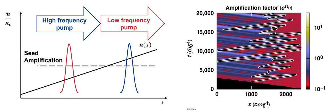
A large bandwidth mitigates the transient gain enhancement of SRS
