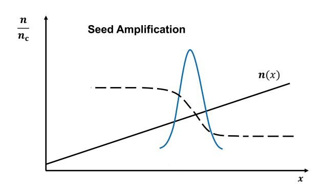
A large linear gain can generate Langmuir waves capable of trapping electrons, initiating kinetic inflation\*
