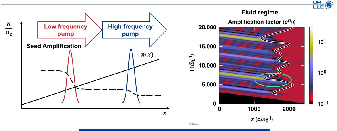
This transient gain enhancement requires a delicate balancing of plasma and pump parameters:\*  $\frac{\mathrm{d}\Delta\omega}{\mathrm{d}t}=-\frac{\omega_\mathrm{p}c}{4L_\mathrm{n}}$
