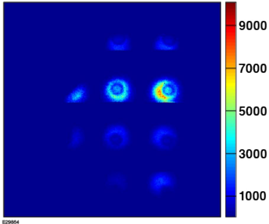
Only six images are usable on this shot due to misalignment of the XRFC and parallax
