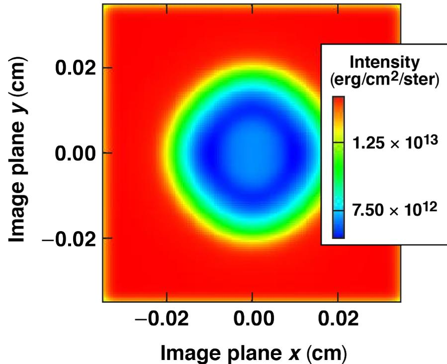
A small  $\ell = 4$  perturbation can be seen in the simulated radiograph at 3 ns
