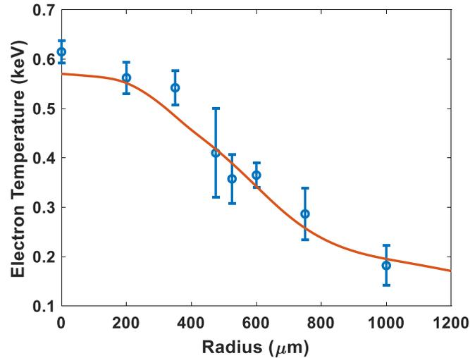
$$k_B T_e = \left( \frac{5 r_0^2 n_e Z^2 e^8 \ln(\Lambda)^2 \omega_p^2}{4 c 3.2 \cdot 72 \pi^3 \epsilon_0^4 \omega_0^2} I \right)^{1/5}$$
