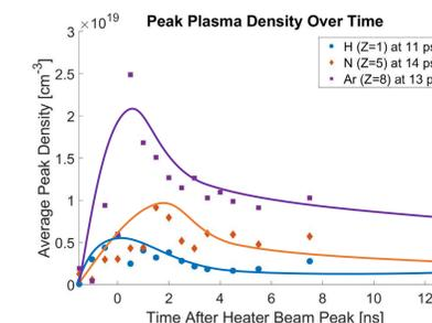
Results indicate higher-Z elements reach expansion velocities larger than that of lighter elements. This leads to sufficiently large temperatures above 100 eV necessary to mitigate IIR, filamentation, and spontaneous Raman scattering.
