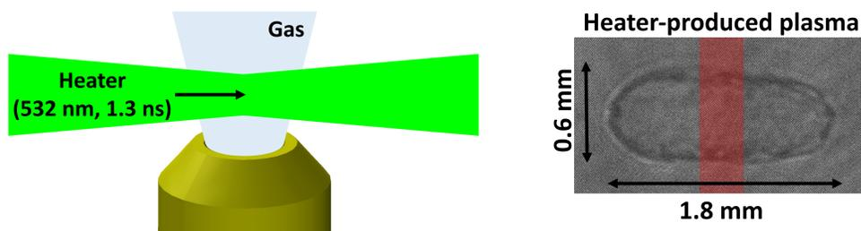
A SID4 (four-wave shearing interferometer device) measures plasma density and size at different delays after the heater beam. Measurements of plasma shape and density are averaged over the region indicated in red. It should be noted that this method is limited by the amount of light absorbed by the plasma as well as shot-to-shot phase modulations in the probe beam.
