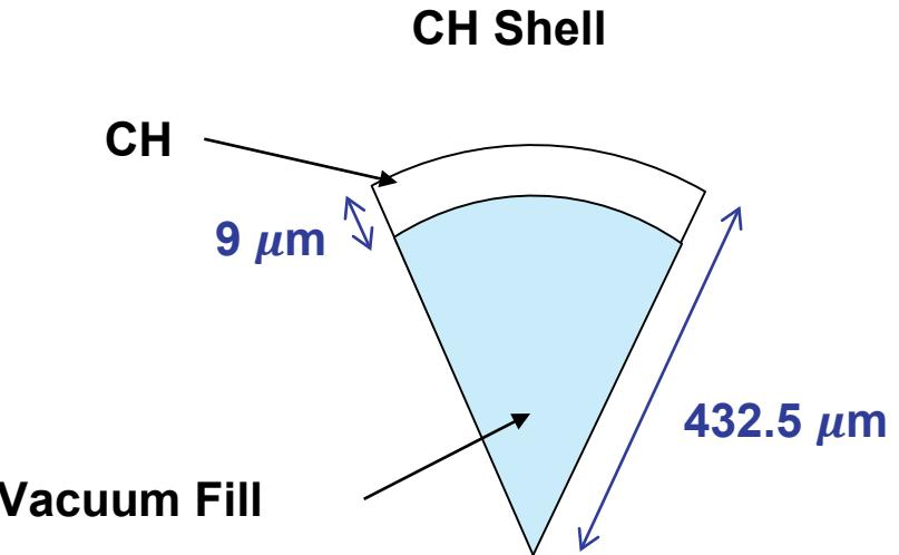
This work will focus on 9  $\mu\text{m}$  thick CH shells with an 865  $\mu\text{m}$  outer diameter and a vacuum fill
