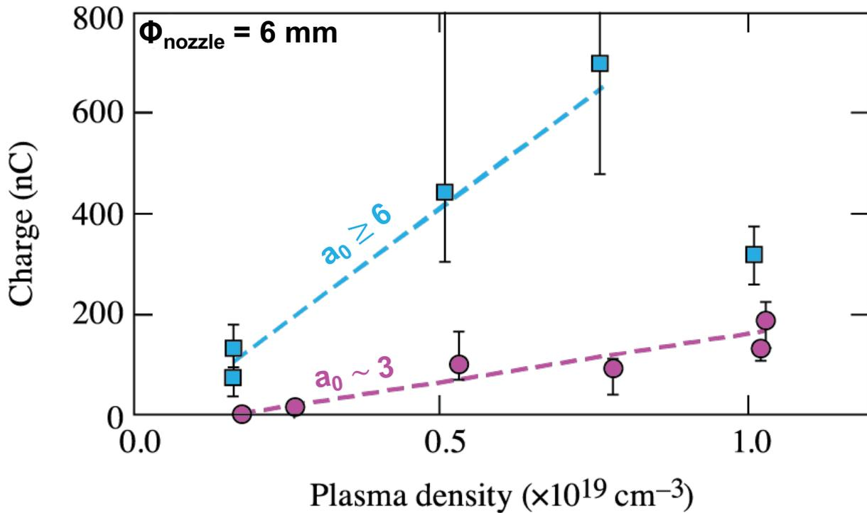
Electron beams with charges up to  $707 \pm 429/224 \text{ nC}$  were measured
