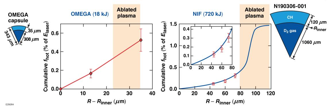
These results support validity of hydro-scaling in warm implosions, though hot electron attenuation in the outer ablator is important and will have to be accounted for in cryogenic implosions with ablated DT
