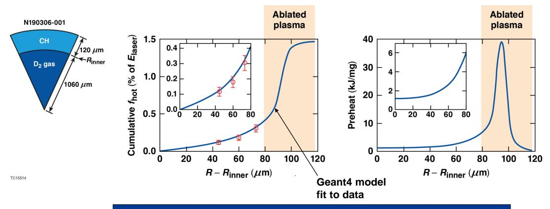
This level of preheat is close to ~0.15% limit for direct-drive ignition designs; Si layers have been found to reduce preheat by ~2x
