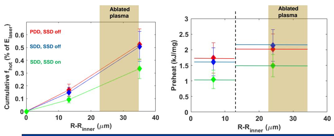
Results are insensitive to polar drive (PDD) vs. symmetric drive (SDD) illumination, but are affected by laser beam smoothing (SSD)
