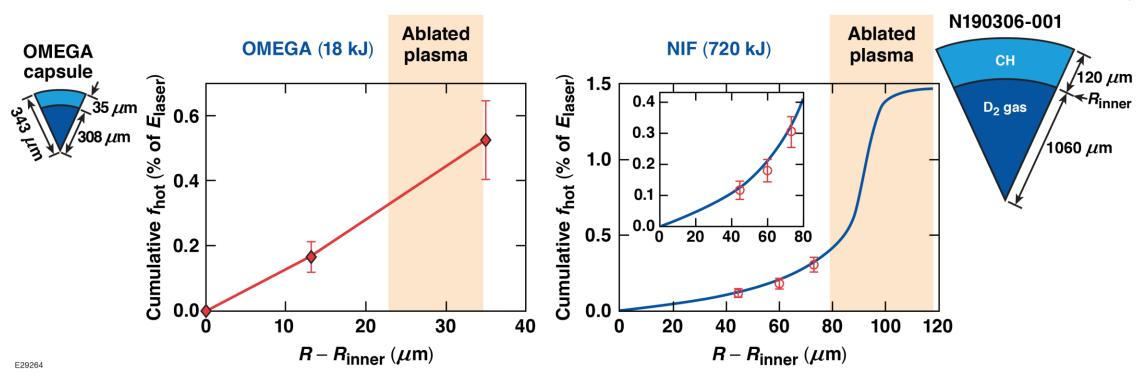
Hypothesis: higher ablated-plasma ρL and SRS hot electrons on NIF generated at larger radius than TPD on OMEGA
