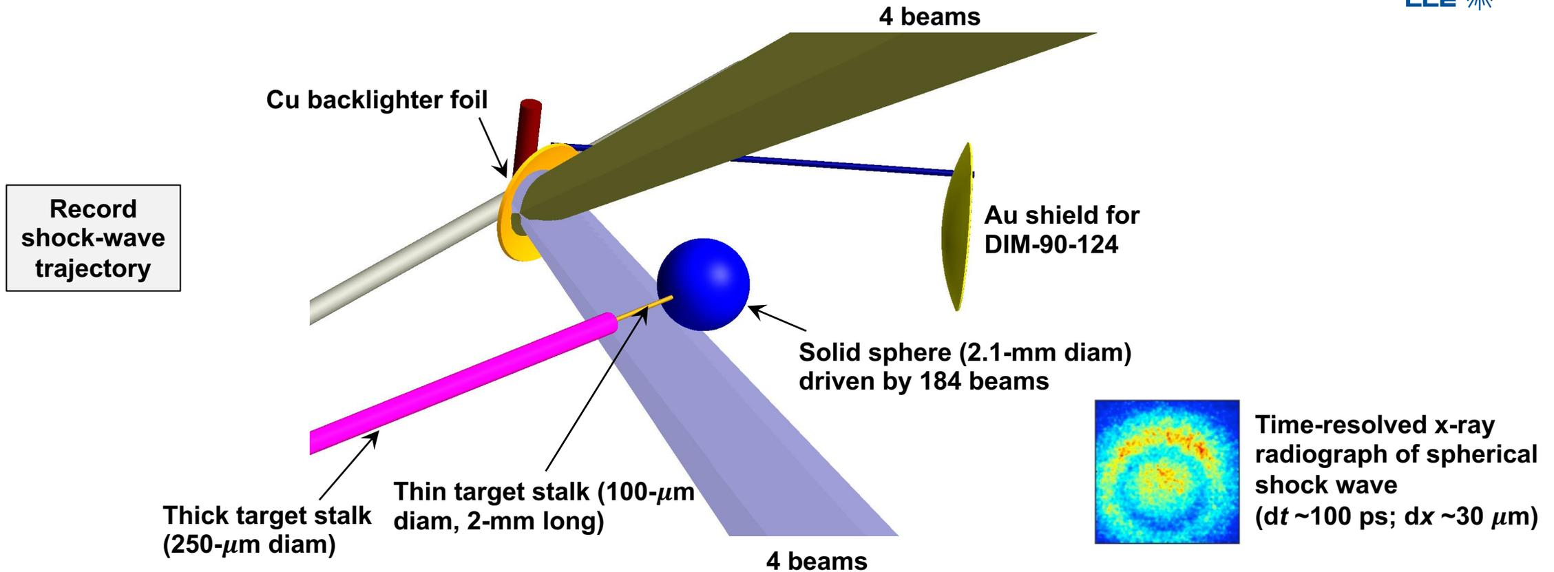
Solid spheres offer the advantage of quantifying energy coupling without the challenges from hydrodynamic instabilities of thin-shell implosions or kinetic effects in exploding pushers.
