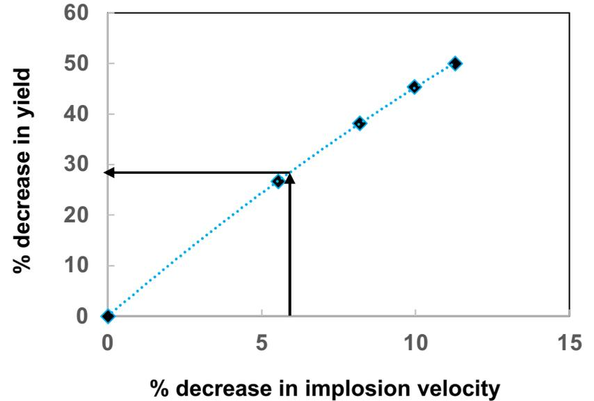
~6% reduction in implosion velocity, delays bang-time by ~ 50 ps and reduces yield by only ~30%
