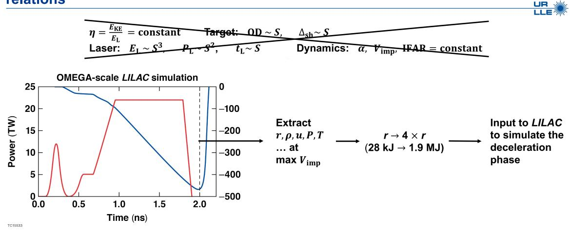
Simulations covered a large parameter space, with 800 < OD ( $\mu$ m) < 1060, 2.5 <  $\alpha$  < 8, and 230 <  $V_{imp}$  (km/s) < 540.
