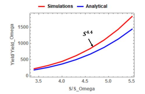
Simulations suggest a faster 1-D no- $\alpha$  yield scaling compared to analytical scaling relations.
