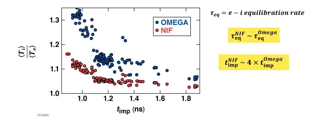
Scaled NIF implosions have more time for ions to lose energy to electrons; therefore,  $T_i$  and, consequently yield scaling, vary as a functions of implosion time.
