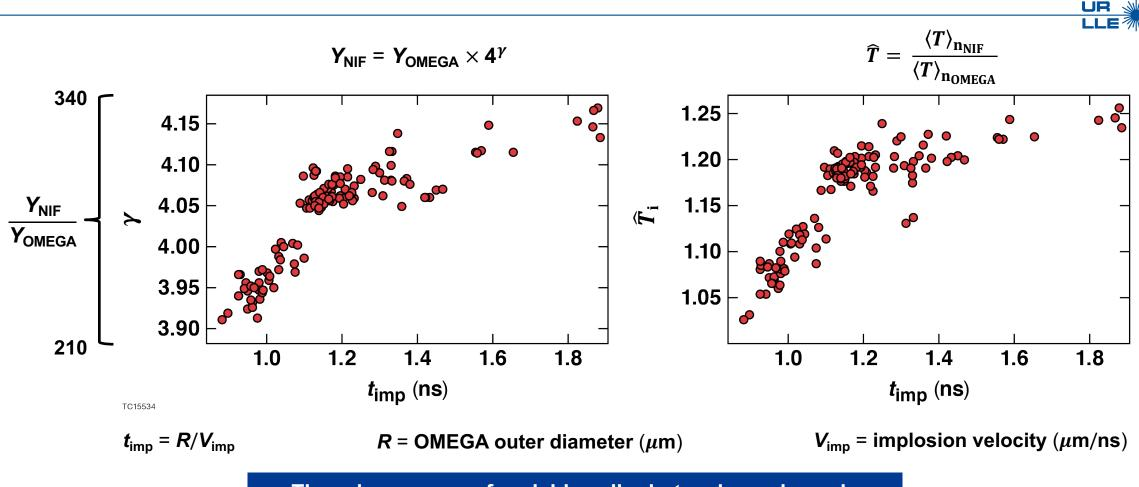
The primary cause for yield scaling's  $t_{imp}$  dependance is the variation in ion temperature scaling with implosion time.
