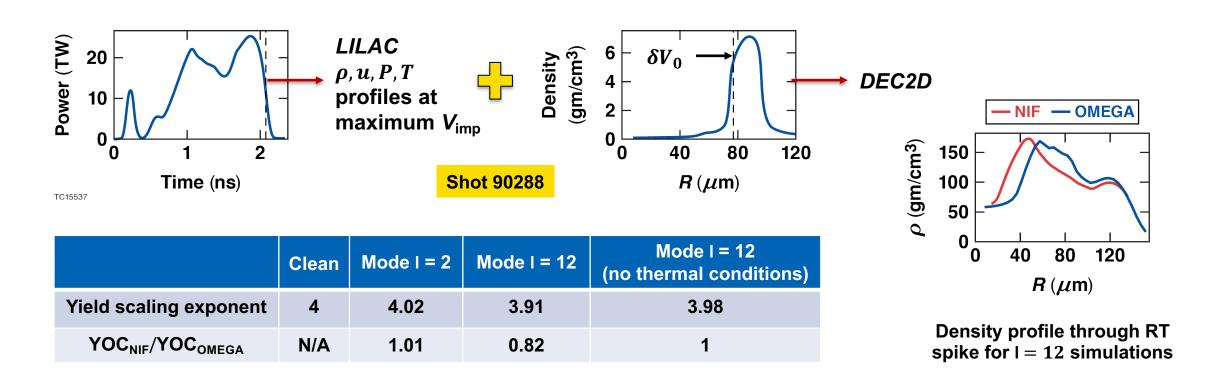
\*The RT instability for I ~ 12 in scaled NIF implosions experiences lower ablative stabilization (higher growth rates) because ablation velocity does not scale hydrodynamically; instead,  $V_{abl} \sim R^{-0.5}$ .
