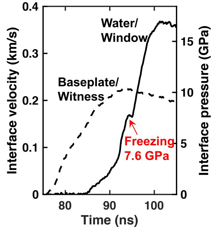
VISAR: velocity interferometer system for any reflector
