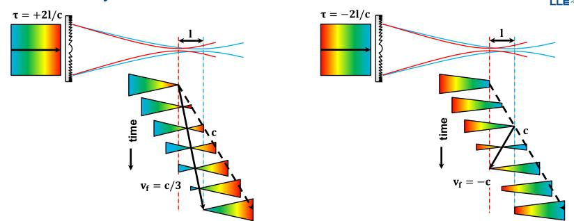
The chirp of the pulse determines the time at which color reaches focus, resulting in a peak intensity with a dynamic trajectory
