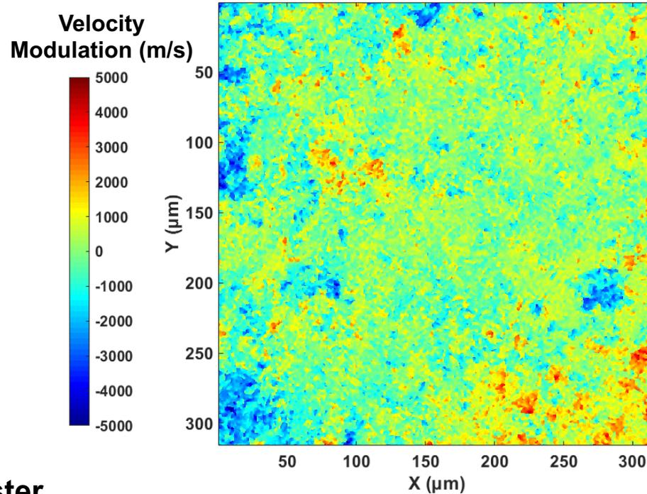
Imprinted shock front modulations from a single OMEGA beam
