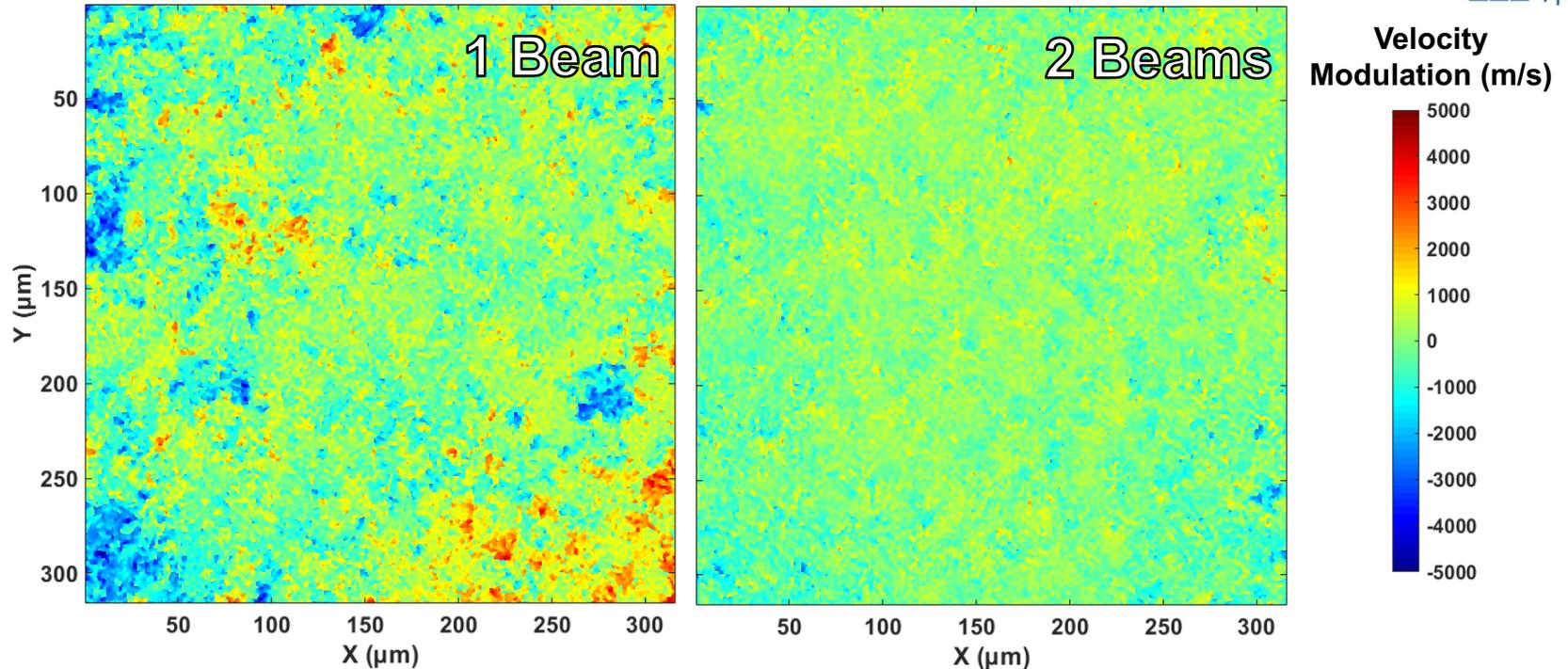
**Addition of second beam shows clear reduction of imprinted modulations**
