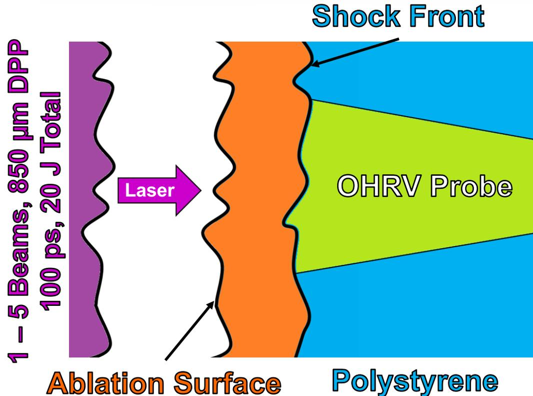
OHRV measures distortions closer to the initial laser imprint seed than x-ray radiography
