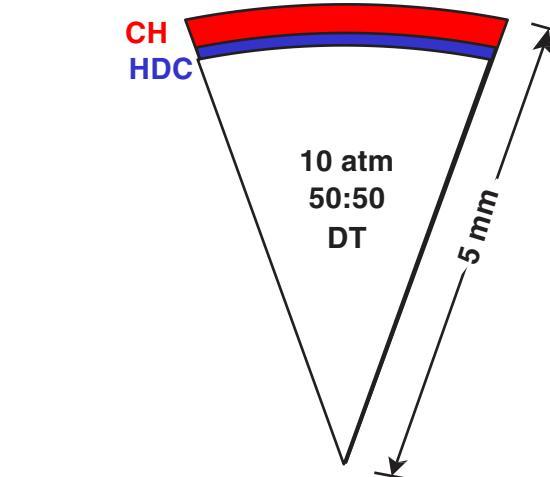
A CH overcoat will enable fielding a contoured HDC capsule
