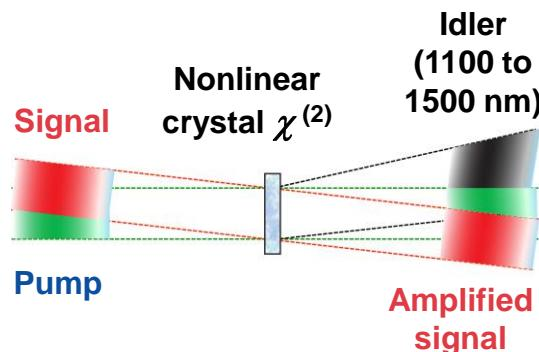
Novel co-linear OPA proposed for efficient amplification
