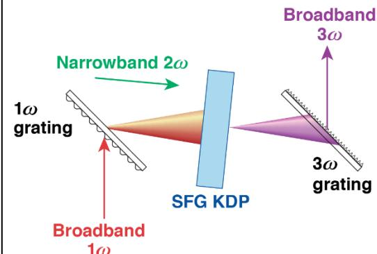
Efficient broadband frequency conversion (1 $\omega$  to 3 $\omega$ ) by SFG with narrowband 2 $\omega$
